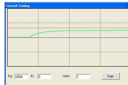
Figure 23: Kp=2604, Ki=0 (poor performances)
