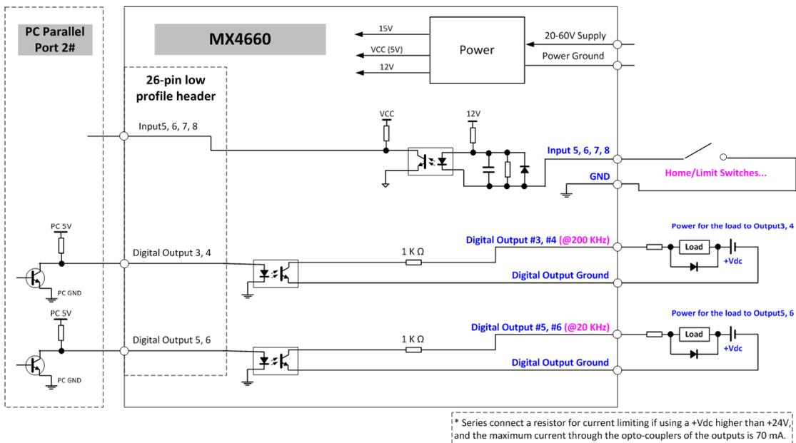
Figure 17 Connecting digital output3, 4, 5, 6
