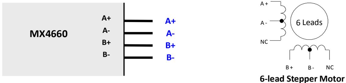
Figure 6 Connecting a 6-lead stepper motor in half-coil
