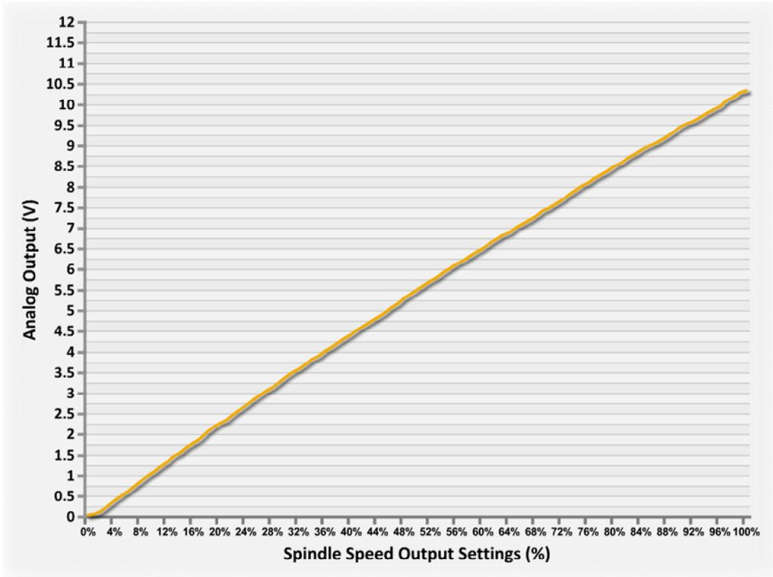
Figure 19 Spindle output & analog output of the MX4660
