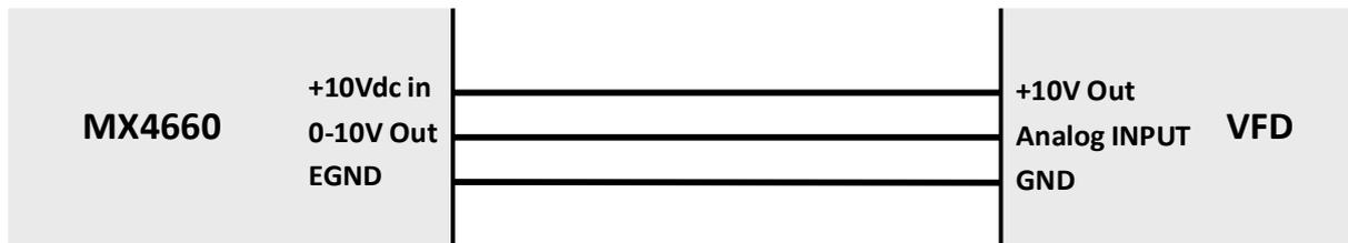
Figure 18 Connecting a VFD to the MX4660
