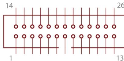
Figure 23 Pin assignments of the 26-pin low-profile connector
