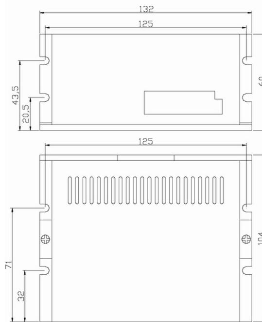
Figure 1: Mechanical specifications
