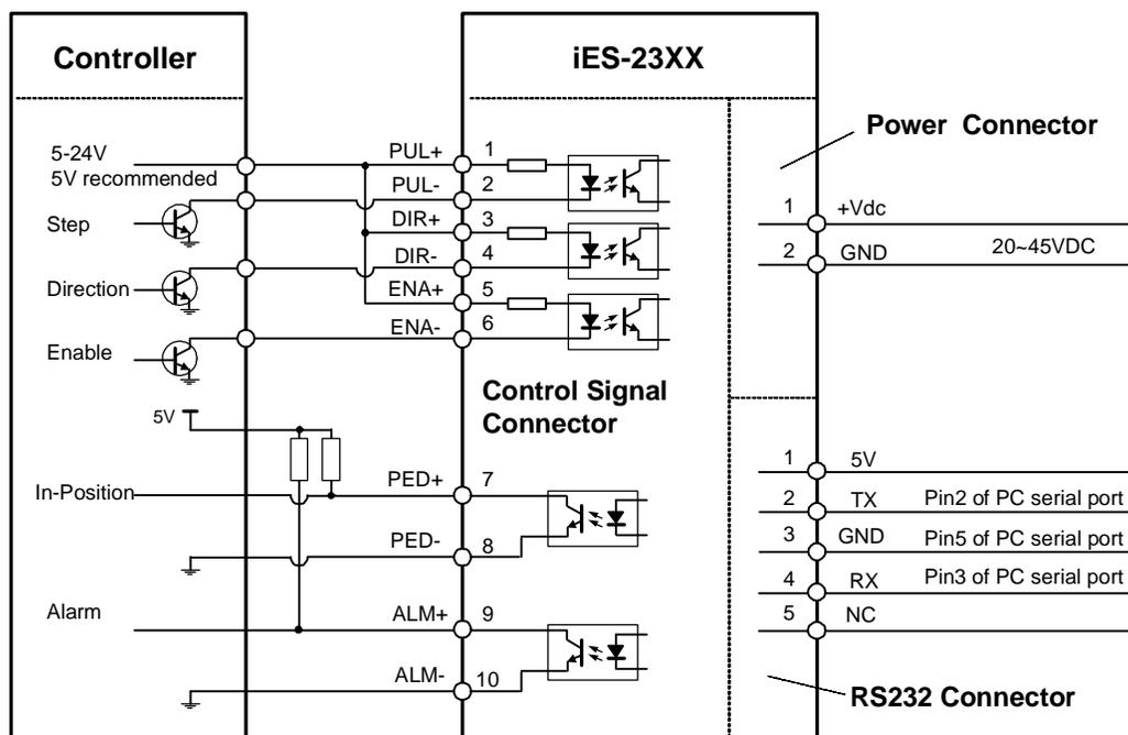
Connect iES-23XX to controller of sinking output
