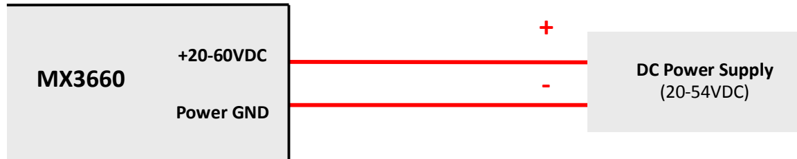
Figure 4 Power supply connections
